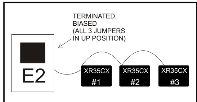
Figure 18-2 - MODBUS Networking
