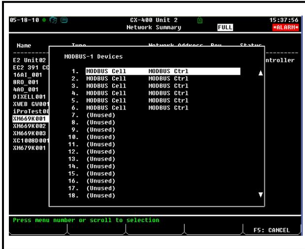
Figure 18-6 - List of MODBUS Devices
