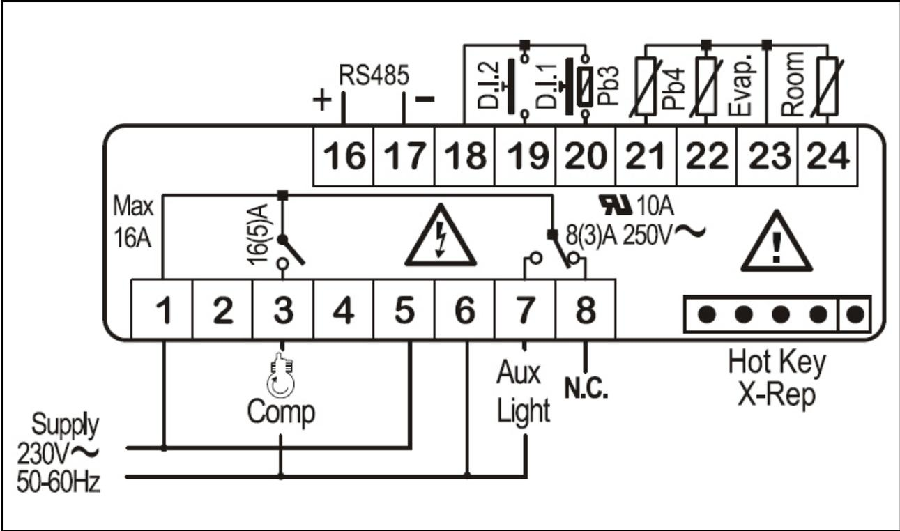
Figure 16-1 - XR35CX Connections
