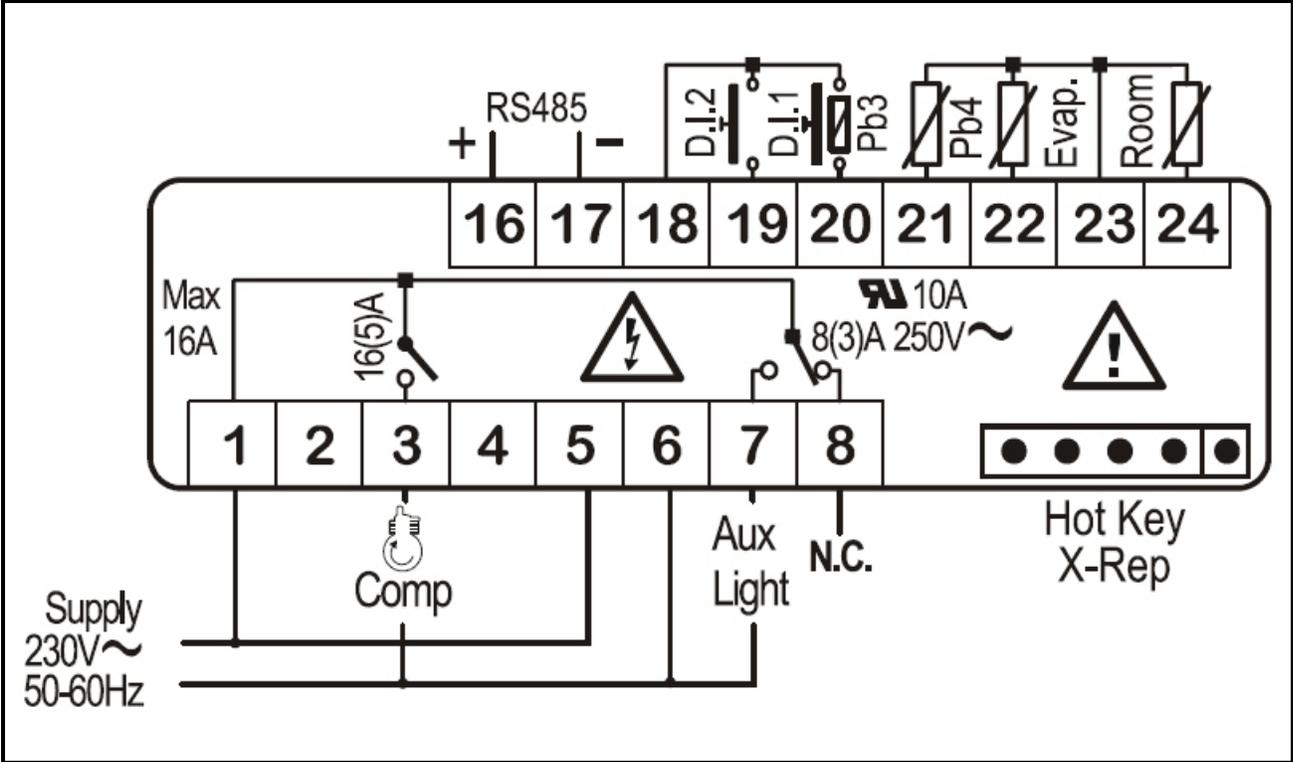
Figure 16-1 - XR35CX Connections
