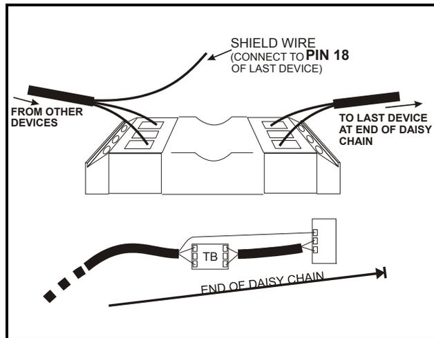
Figure 18-8 - MODBUS Termination Block (P/N 535-2711)
