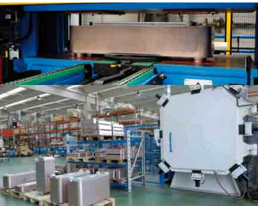
In the new fully automatic test machine the brazed plates heat exchangers are tested for a working pressure up to 30 bar (45 bar for the H version).
