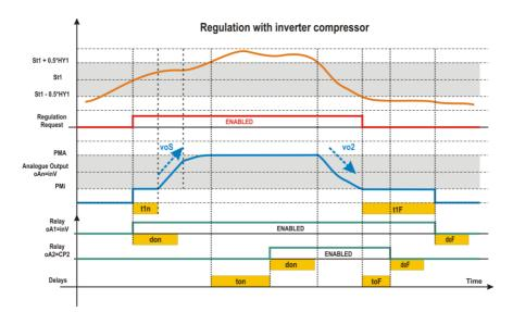
It is possible to drive inverter with control signal of frequency or voltage (0-10 V DC) type. **NOTE:** the analog output is not configurable. It may be frequency or voltage type depending on the hardware.
